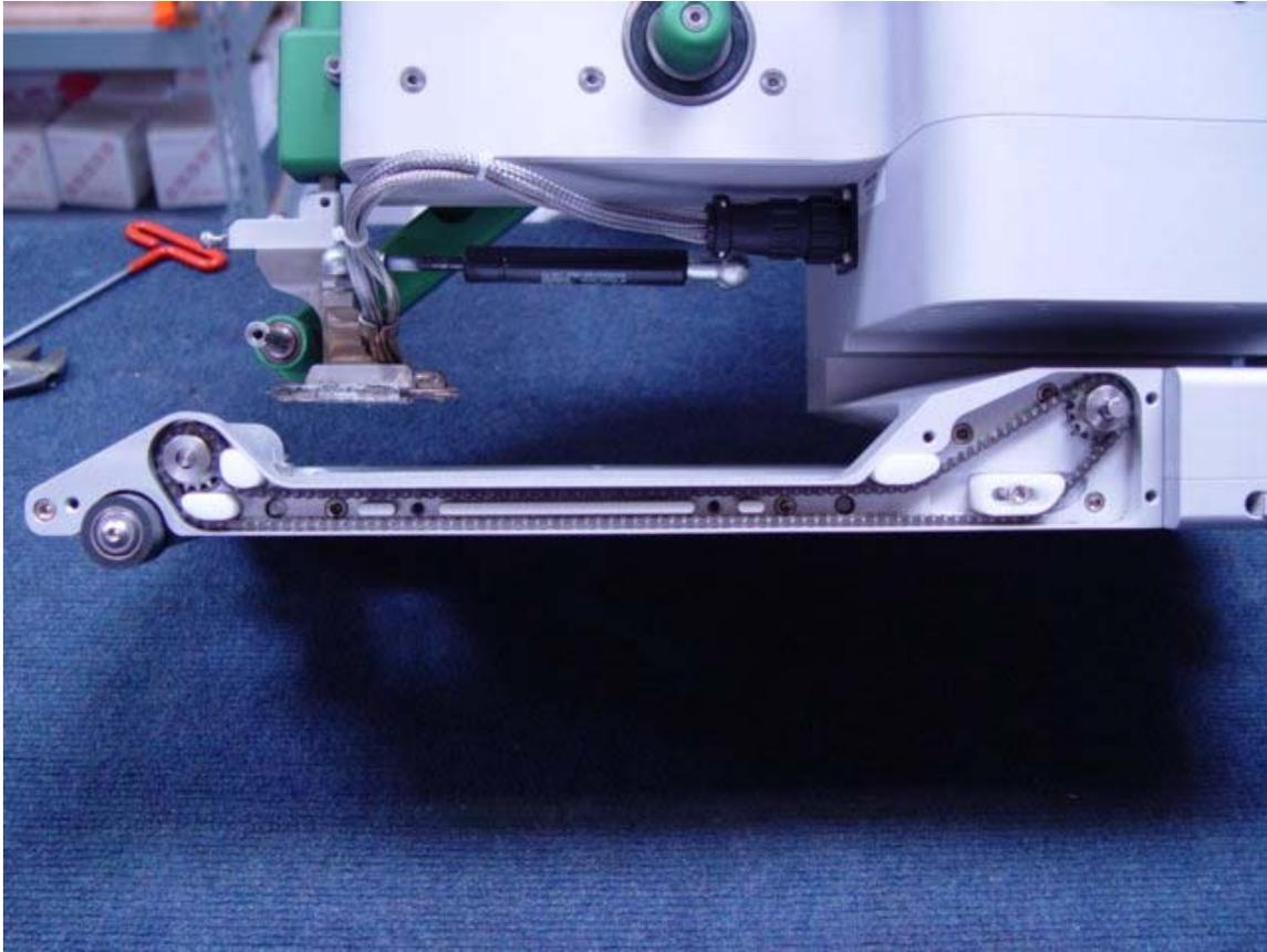
Lower final drive chain part # 300 221 forward rotation anti-clockwise
